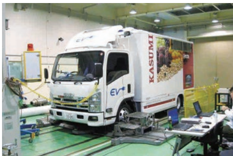
JC08測定風景 Taking JC08 measurements
